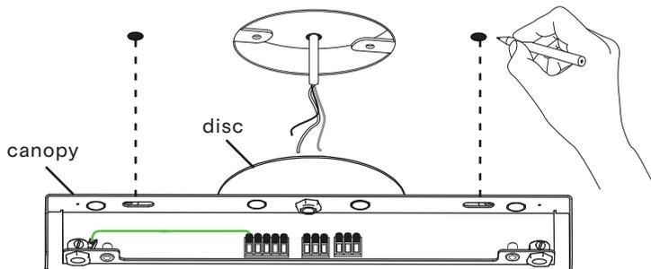
Before marking your anchor points, align the ceiling disc with the center of your junction box. Use canopy as a guide.
