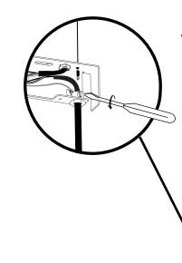
Loosen set screw to adjust wire length. Screw back gently but firmly, when desired wire length is reached.
