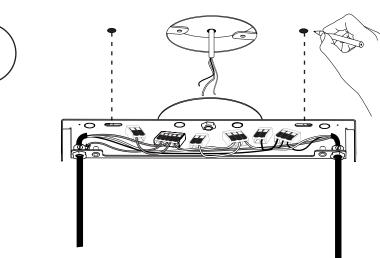
Before marking your anchor locations, align the ceiling bracket with the center of your junction box.
