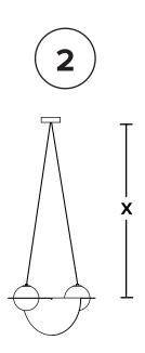
Trim wires to desired length (X). Do not leave a large excess of wires inside canopy. Reconnect them as before. Loosen set screws to adjust wire length. Screw back gently but firmly when desired wire length (X) is reached.
