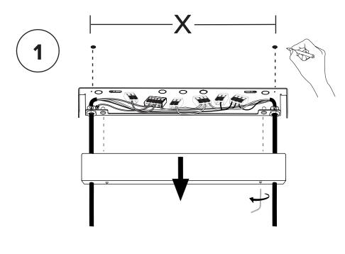
Lower ceiling bracket cover then use the bracket as a guide for your anchor holes. Make sure to use appropriate anchors for ceiling material.
