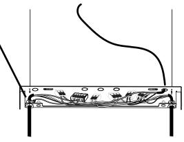
Trim wires to desired length (**X**). Do not leave a large excess of wires inside the canopy. Reconnect them as before. Do this step before installing luminaire to the ceiling
