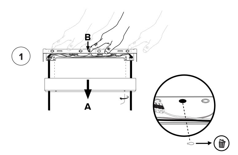
Knockout selected hole depending on desired electrical box alignment.
