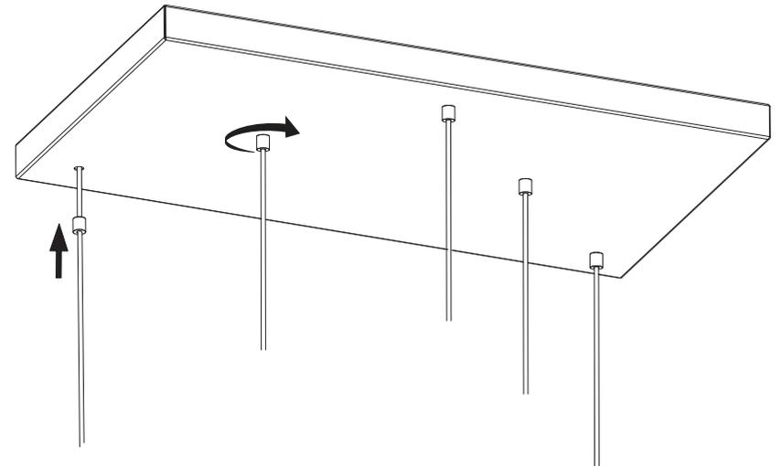
When adjustments are complete, raise the canopy cover and secure it in place by screwing the caps back into place.
