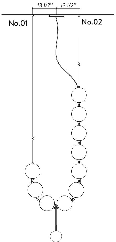
**15** Blocking/support must be included in the ceiling for the installation of the Coco and must support minimum 120lbs. Use appropriate screw (not included)
