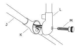
To adjust the Arm angle loosen the Thumb Screw while holding the Arm of the light. Adjust to the desired angle and secure in place by tightening the Thumb Screw.
