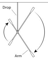
The Hang-Straight hardware allows for the fixture to be rotated and adjusted to hang straight.
