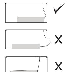
If your wires are too short or too long, unscrew end cap, losen strain relief screws on, pull wires out further while making sure the protective sleeve stays under the strain relief.
